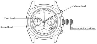
In the case the crown is of the screw-lock type, loosen the screw by turning the crown to the left before operating the crown, and after having returned the crown to the normal position following operation, turn the crown to the right while pushing it in to securely retighten it.
